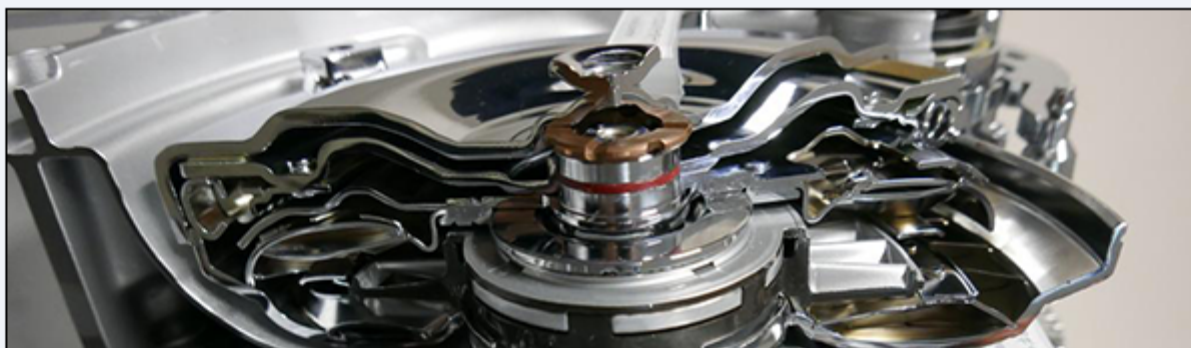
1 - front support, 2 - drive sprocket, 3 - driven sprocket, 4 - oil pump body, 5 - cam ring, 6 - rotor, 7 - oil pump case, 8 - vane. a - inlet port, b - low pressure discharge port, c - high pressure discharge port
