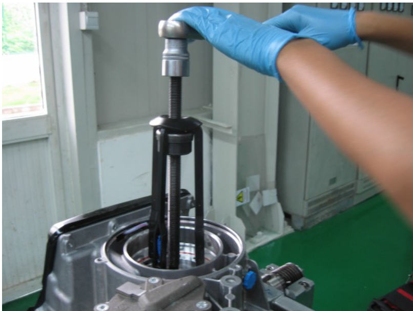
Figure 7-5 Tighten the bolts in the middle to pull out the bearing
