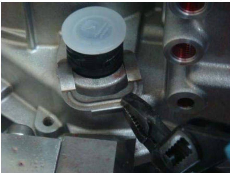
Figure 15-1 Remove the buckle from the main connector.
