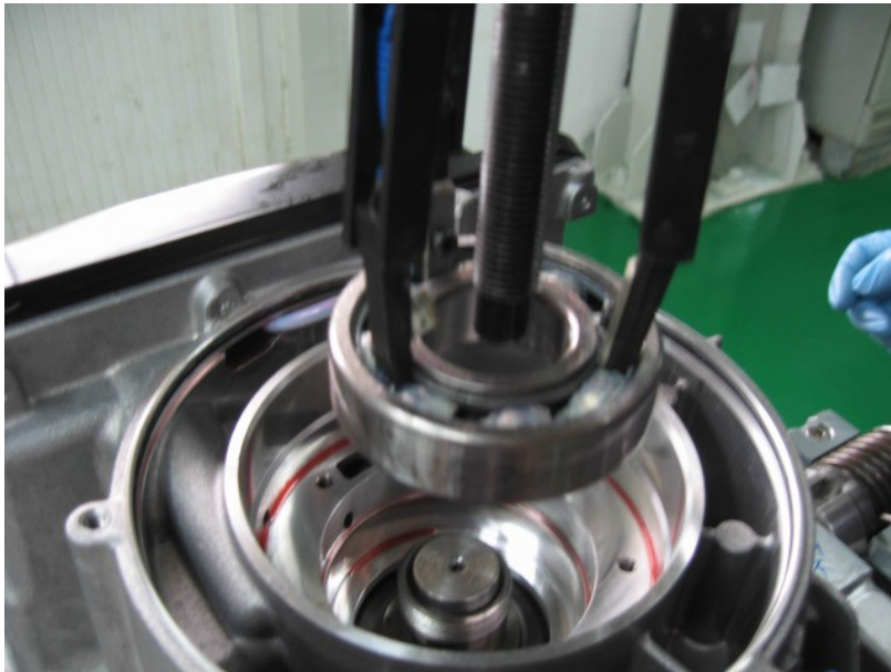
Figure 7-6 Remove the bearing of the driving bevel pulley
