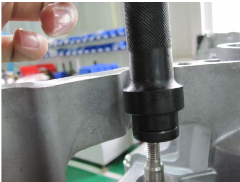
Figure 4-6 Use a special tool (480125) to place the oil seal on the gear selector shaft.
