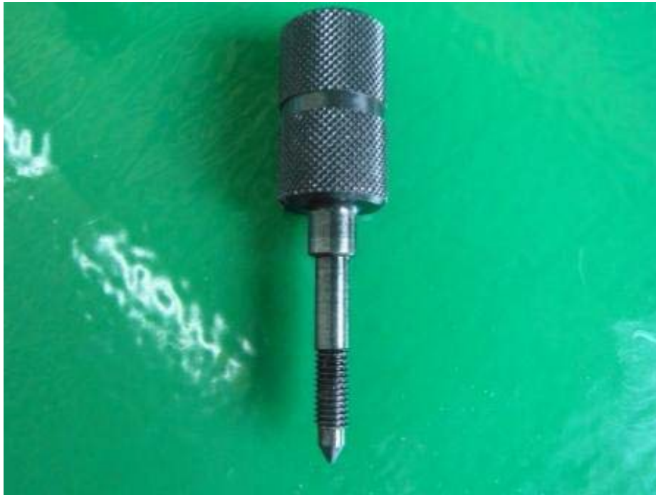
Locating pins of hydraulic control block (drawing 480142)
