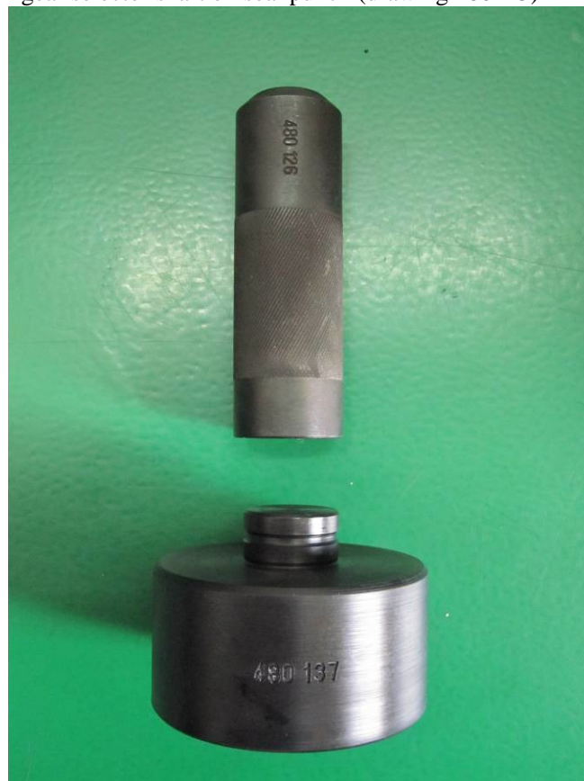
Bearing punch of driving bevel pulley shaft (drawing 480137 + 480126)
