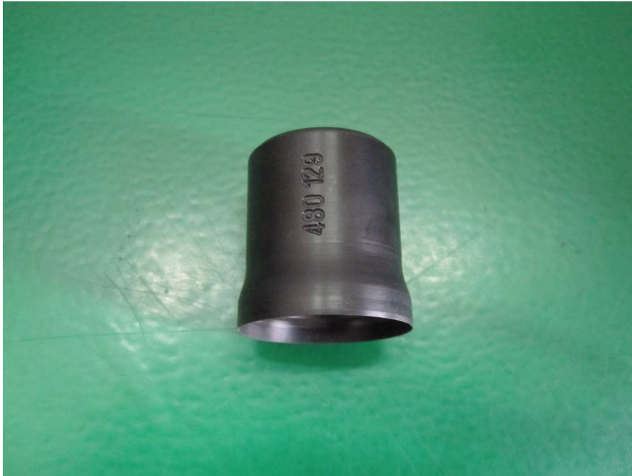
Positioning sleeves of input shaft oil seal (drawing 480129)
