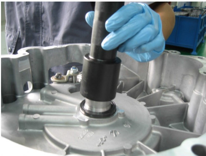
Figure 3-4 Use a special tool to mount the oil seal (480130)
