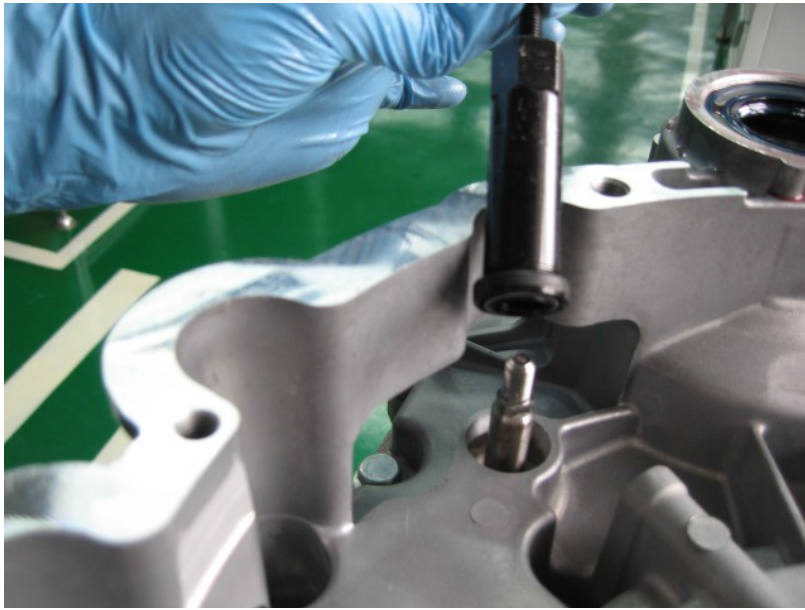
Figure 4-4 Remove the oil seal.
