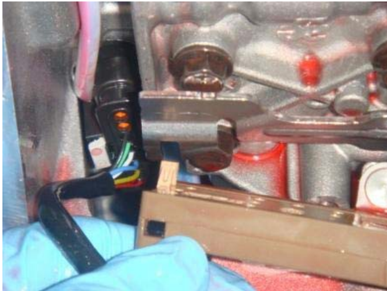
Figure 11-4 Mount the pin correctly on the metal slider.
