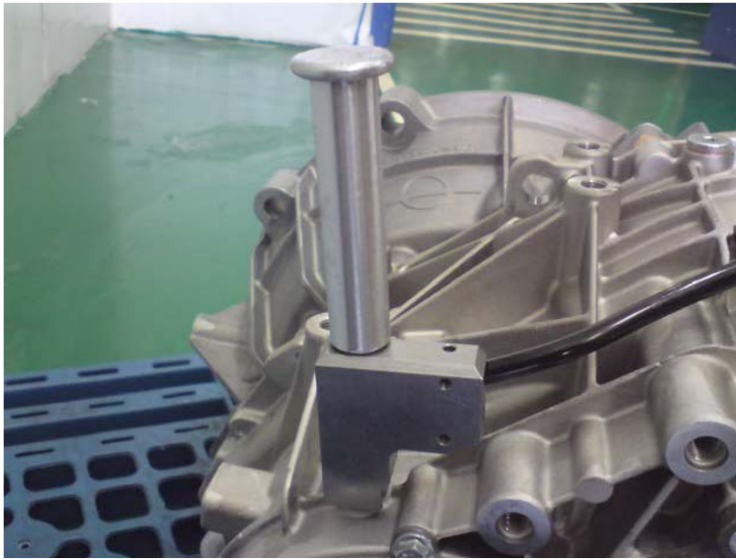
16-2 Install the breather pipe.
