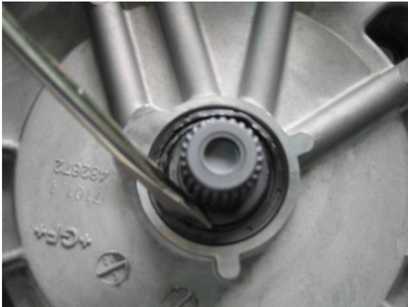
Figure 3-1 Remove the input shaft oil seal.
