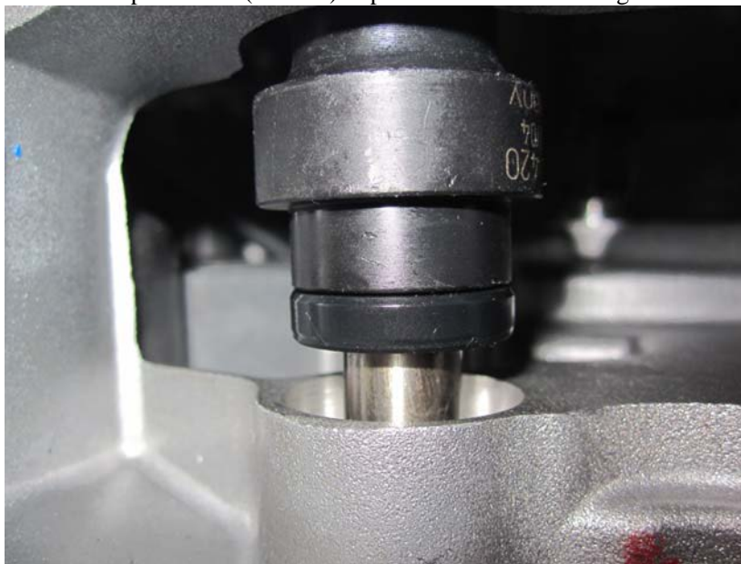
Figure 4-7 Use a hammer to knock the tool (480125) until fully in place.
