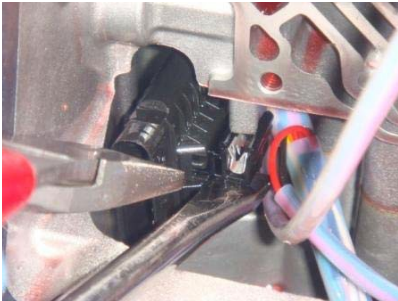
Figure 15-6 Press the driving mode sensor connector on the casing.
