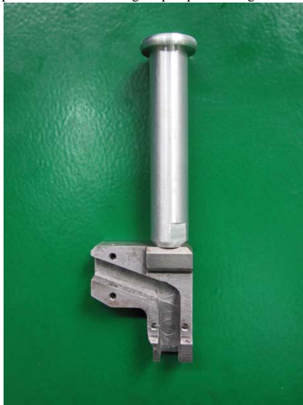
Respirator pipe installer (drawing 480140)
