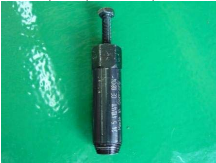
Tool for removing gear selector shaft oil seal (drawing 480127)
