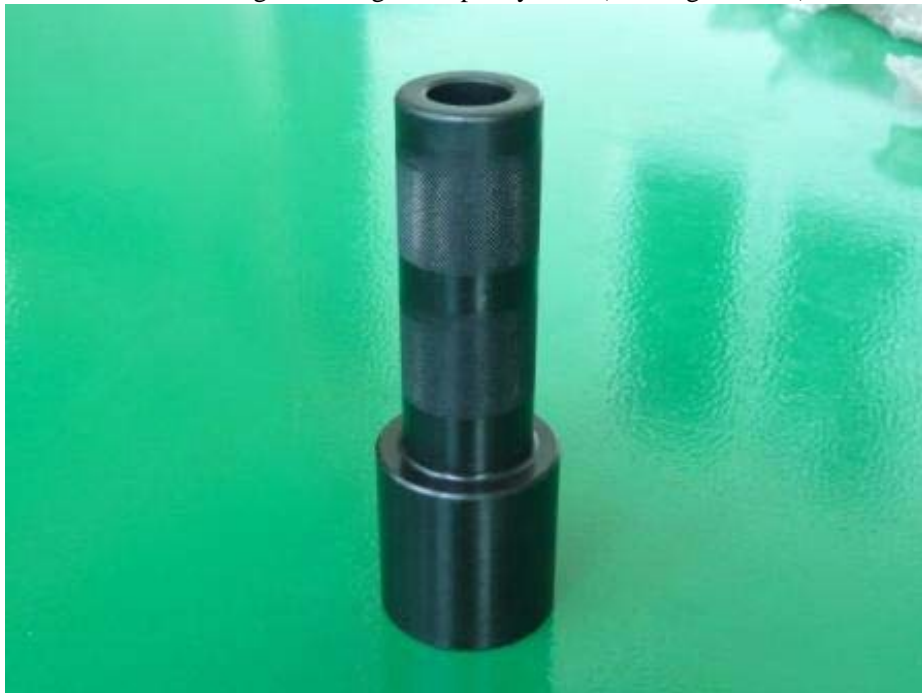
Input shaft oil seal punch (drawing 480130)
