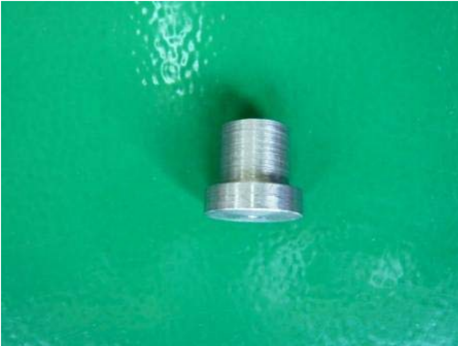
Bearing plug of driving bevel pulley shaft (drawing 480139)
