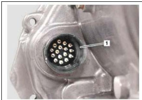
Figure 17 Wiring harnesses on the transmission
