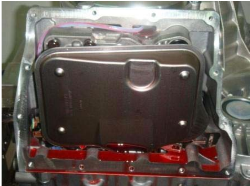
Figure 10-2 Install the filter in place
