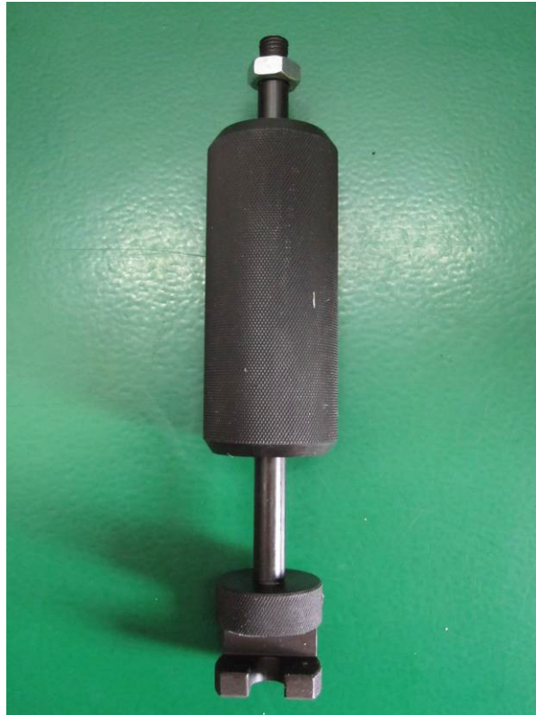
Special tool for removing oil pump (drawing 480141)
