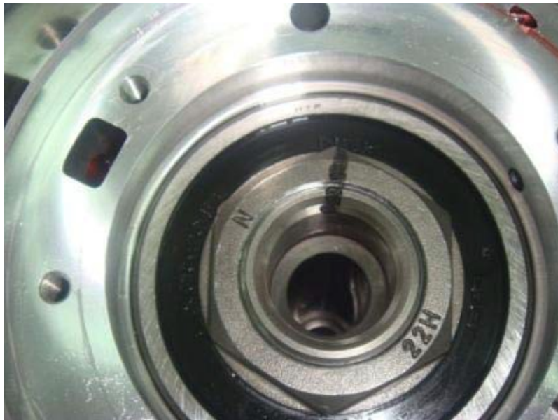
Figure 7-1 Leave marks on the shaft and nuts
