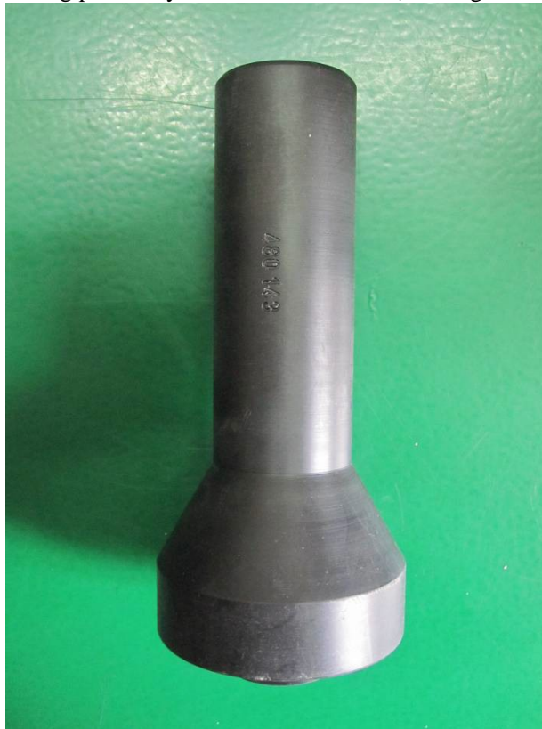
Differential oil seal punch (drawing 480143)
