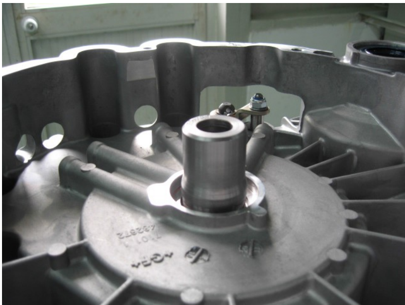
Figure 3-2 Mount the special tool on the input shaft (480129).
