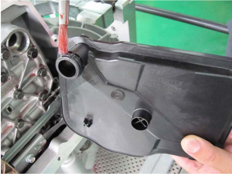
Figure 10-1 Lubricate the O-ring
