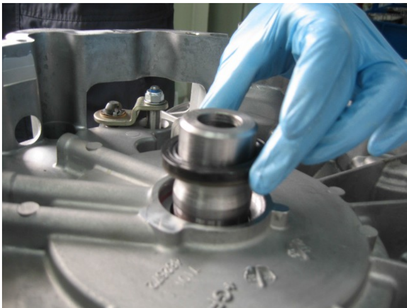
Figure3-3 Press the oil seal downward.
