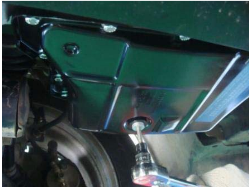
Figure 9-1 Remove oil drain plug
