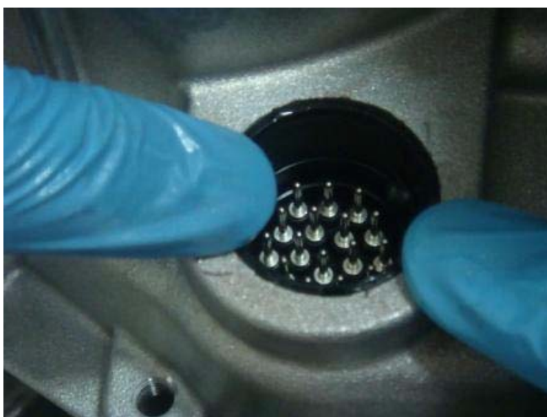
Figure 15-2 Press the main connector into the transmission.
