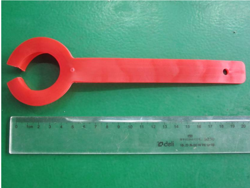
Half shaft installer (drawing 48154)
