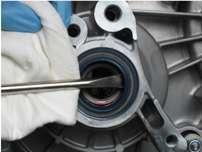
Figure 2-1 Remove the oil seal.
