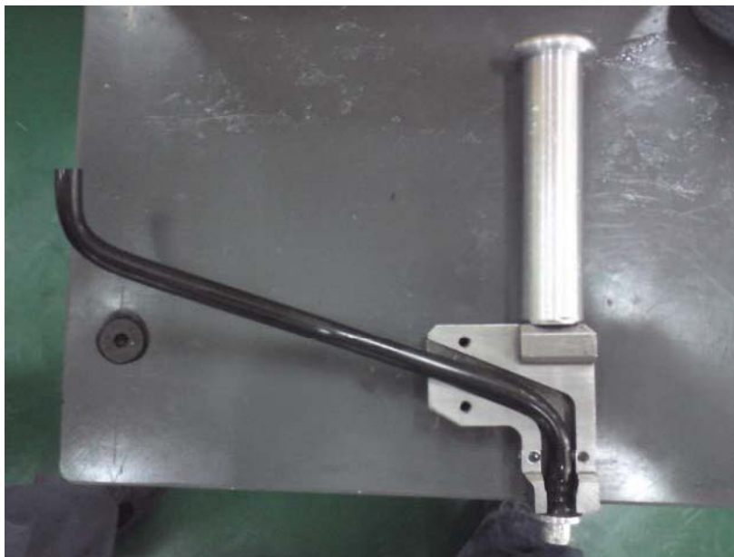
16-1 Put a new breather pipe in the tool.
