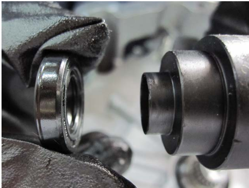
Figure 4-5 Slide the oil seal around the tool.
