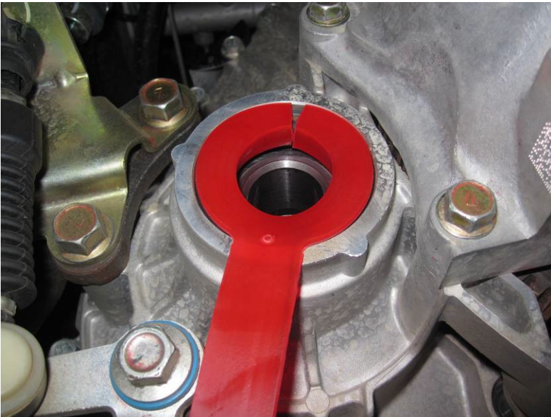
Figure 1-2 Installation by means of the special tool 480145
