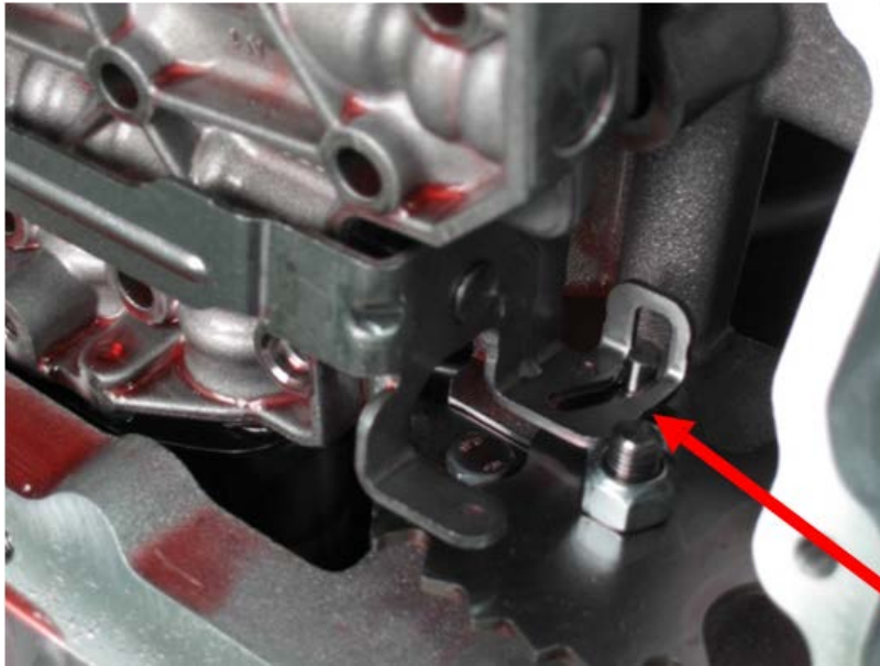
Figure 12-5 The tie rod of the clutch control valve should be correctly located to the positioning pins on the shifting cam.
