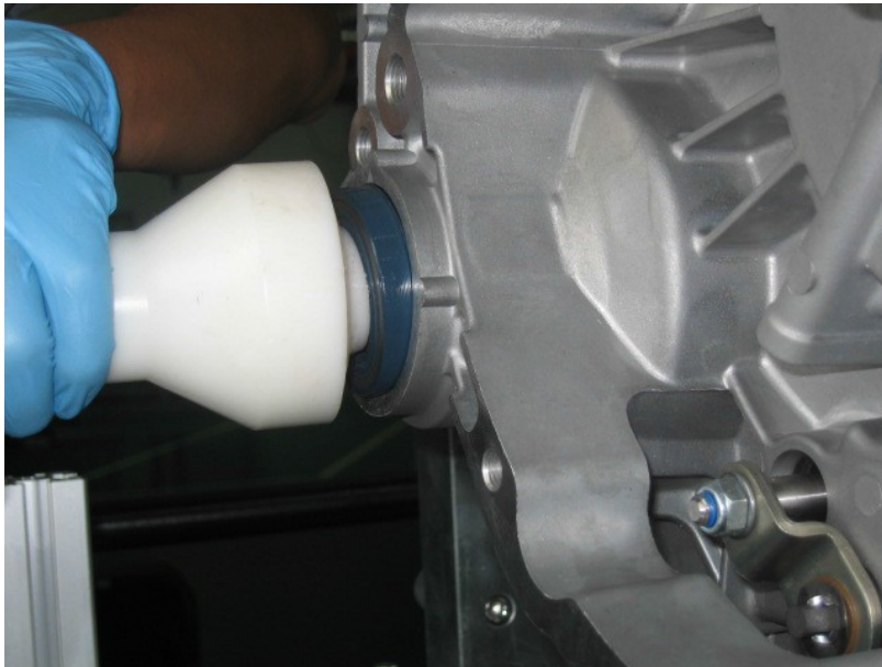
Figure 2-2 Use a special tool to install a new oil seal.
