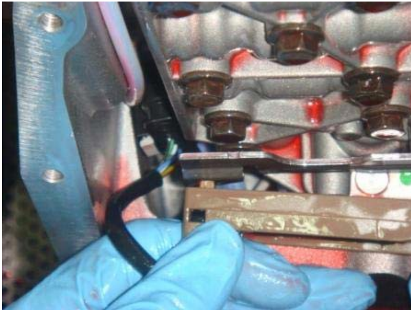
Figure 11-2 Press the sensor downward and pull it out.
