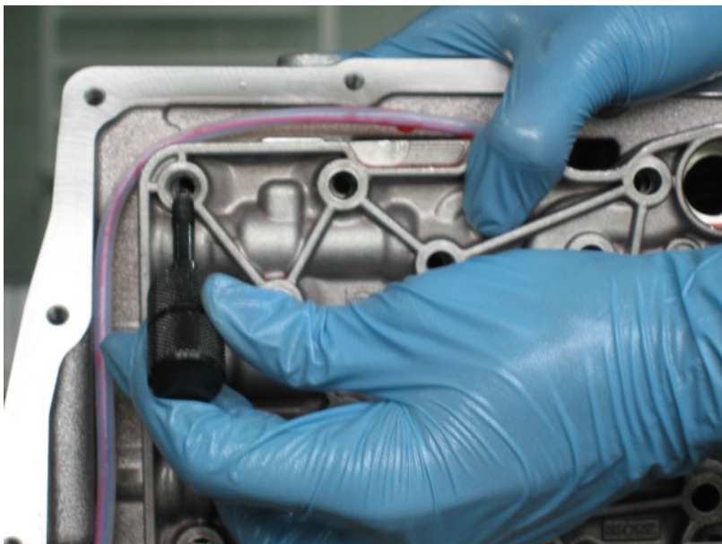
Figure 12-6 Use a special tool (480142) to fix the hydraulic control block.
