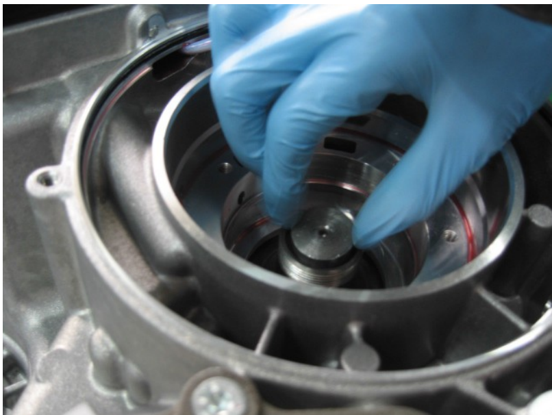
Figure 7-3 Put the special tool on the shaft (driving bevel pulley plug 480139)
