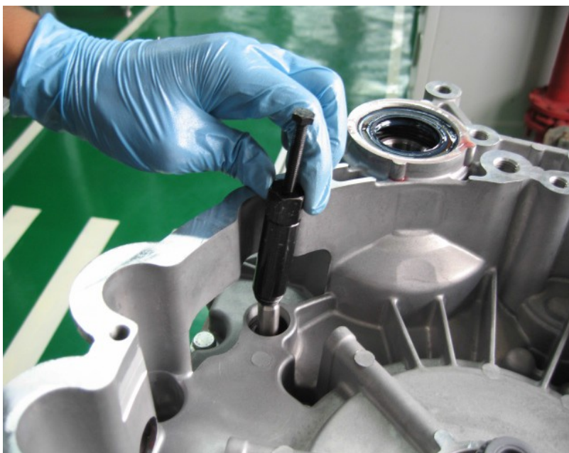
Figure 4-1 Place the special tool (480127) on the gear selector shaft.
