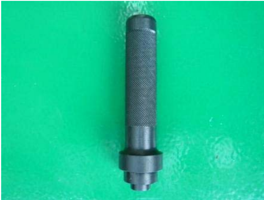
gear selector shaft oil seal punch (drawing 480125)
