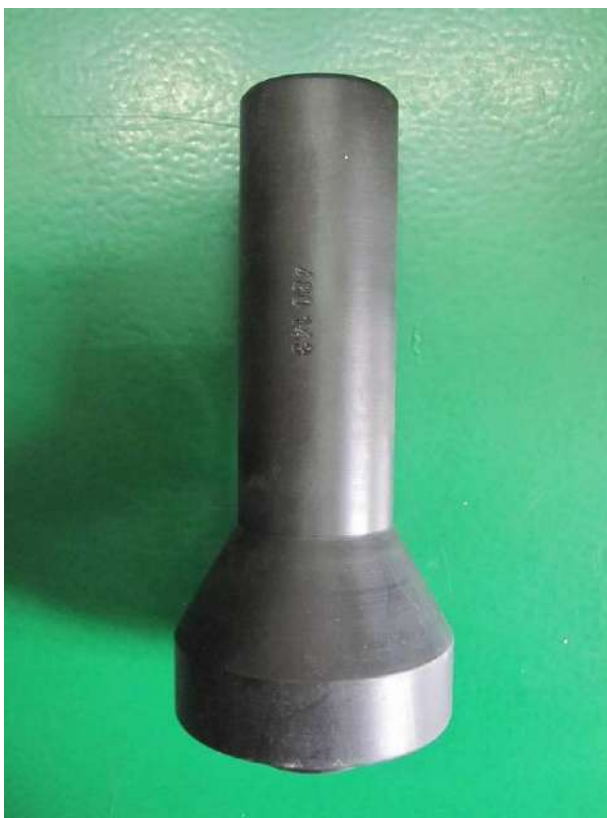
Stamp – oil seal differential (drawing 480143)
