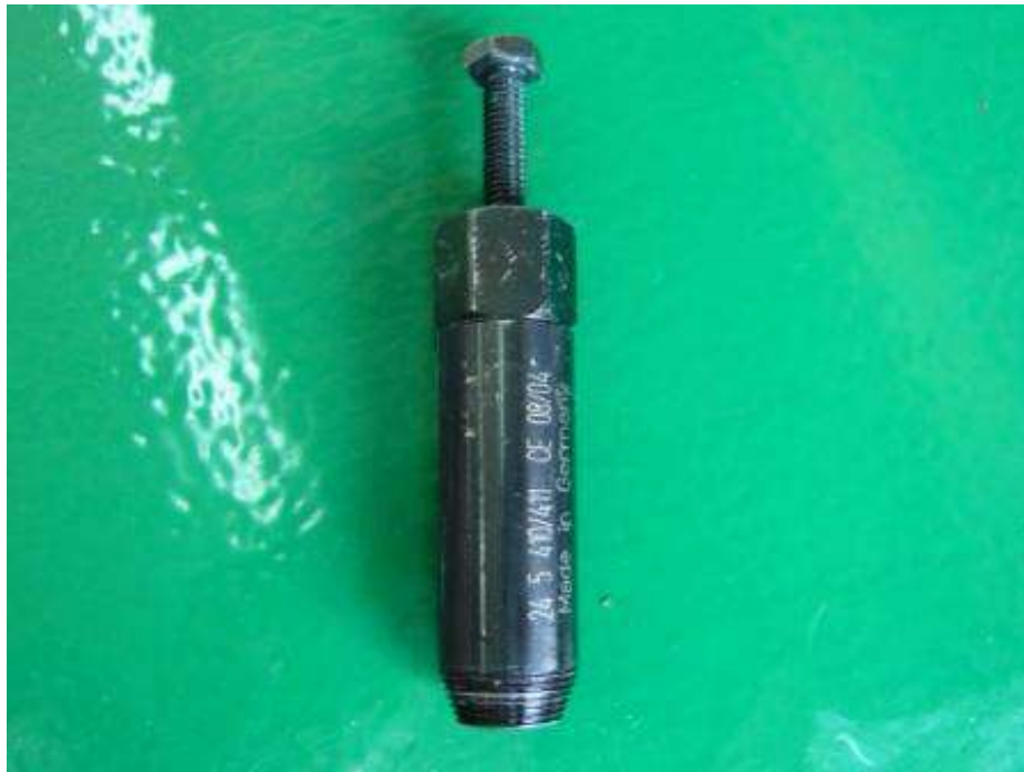
Removing tool – oil seal selector shaft (drawing 480127)
