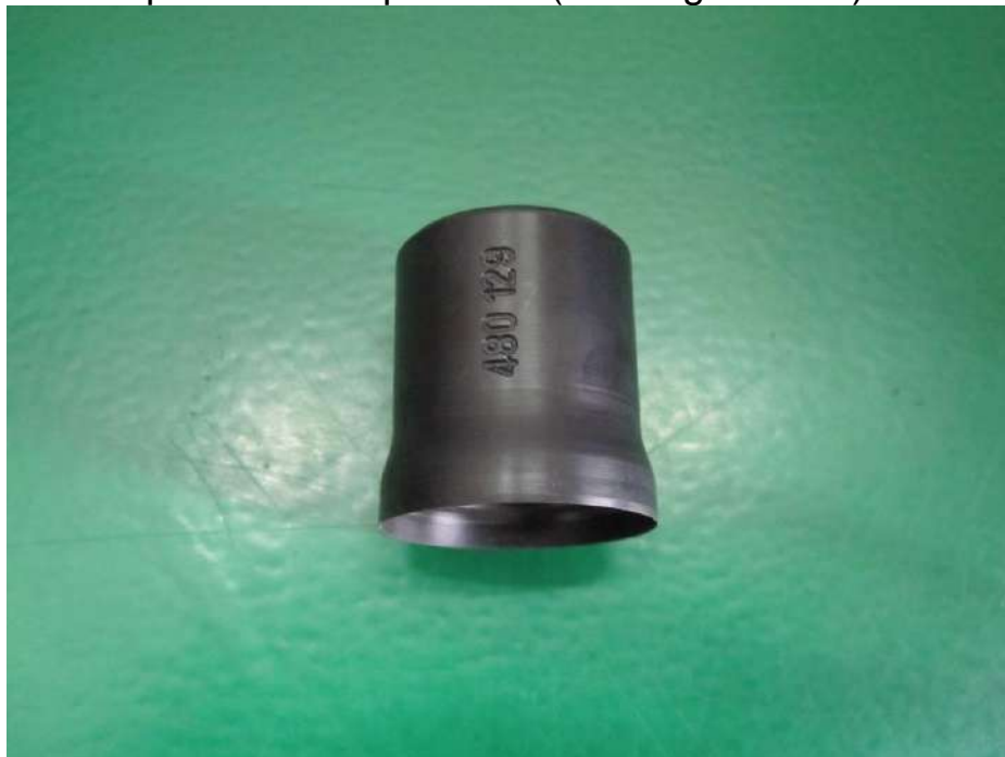
Centering bush – oil seal input shaft (drawing 480129)
