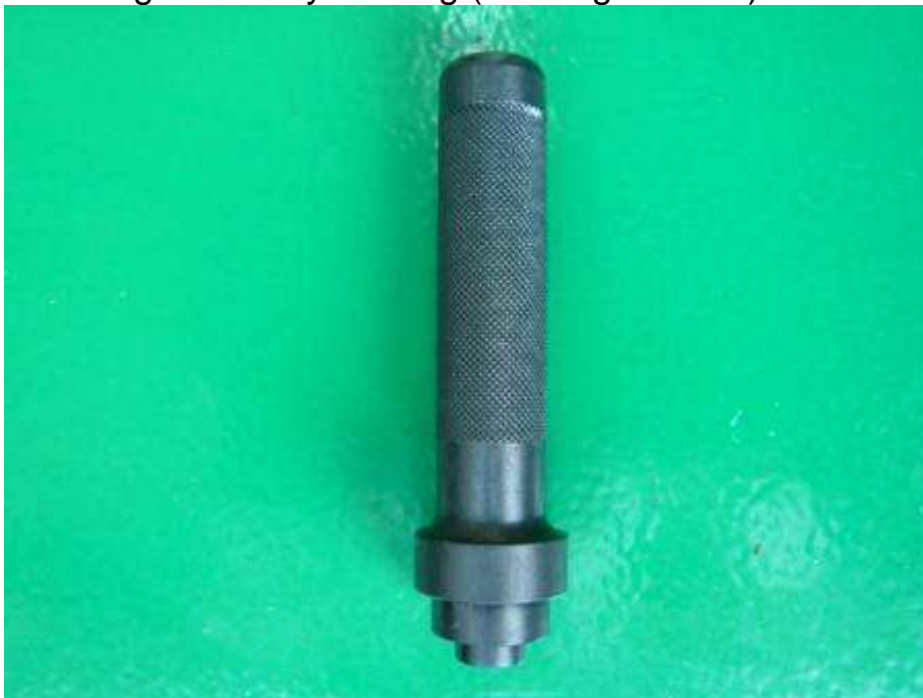
Stamp – oil seal selector shaft (drawing 480125)
