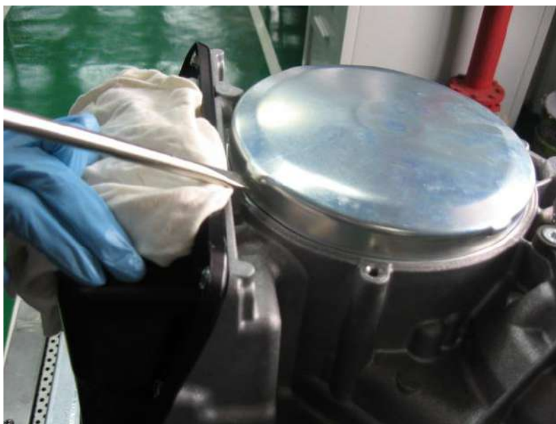
Fig. 5-1: Remove primary cover from transmission
