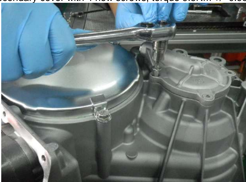
Fig.1 : Take off secondary cover bolt
