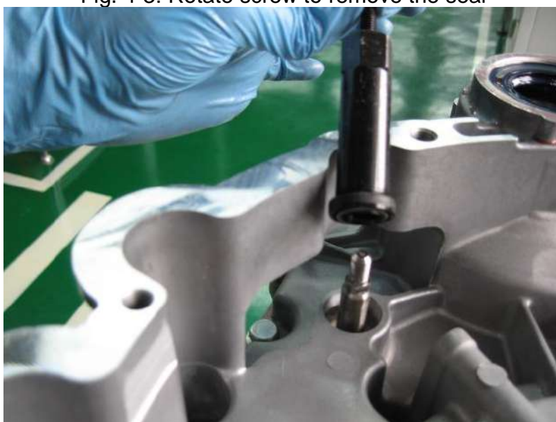
Fig. 4-4: Remove the oil seal
