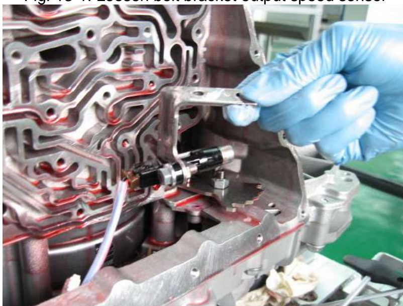
Fig. 13-2: Bracket output speed sensor
