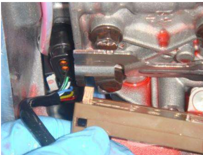
Fig. 11-4: Pin locked in dedicated space of the metal slide
