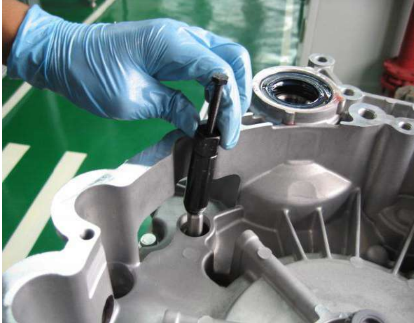
Fig. 4-1: Put special tool (480127) on shaft
