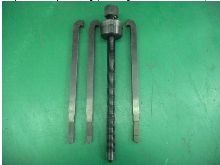
Removing tool – primary bearing (drawing 480136)
