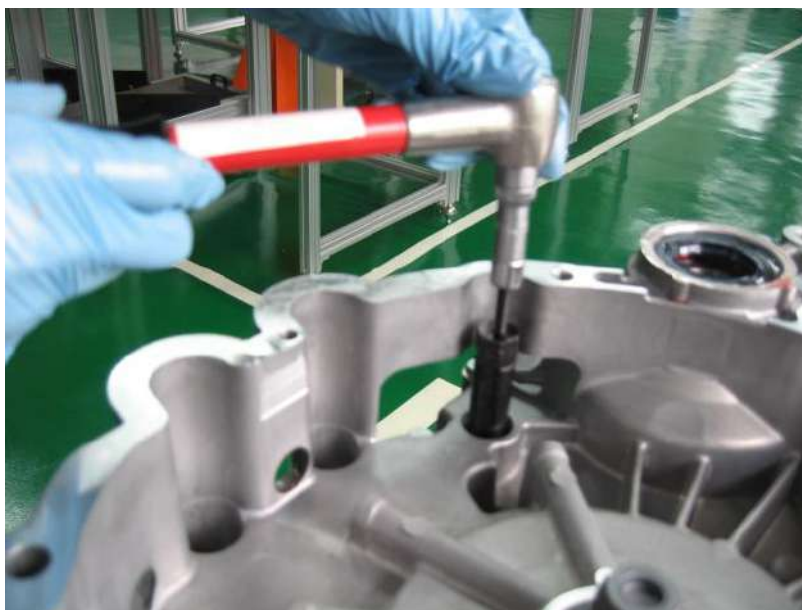
Fig. 4-3: Rotate screw to remove the seal
