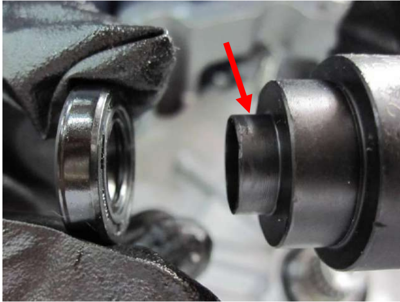
Fig. 4-5: Slide the seal over the special stamp (480125)
