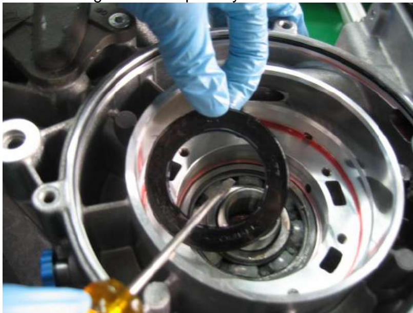
Fig. 7-2: Lever out seal from primary bearing
