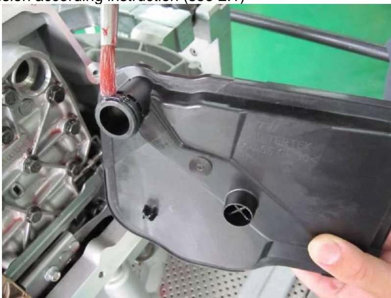
Fig. 10-1: Lubricate the O-ring
