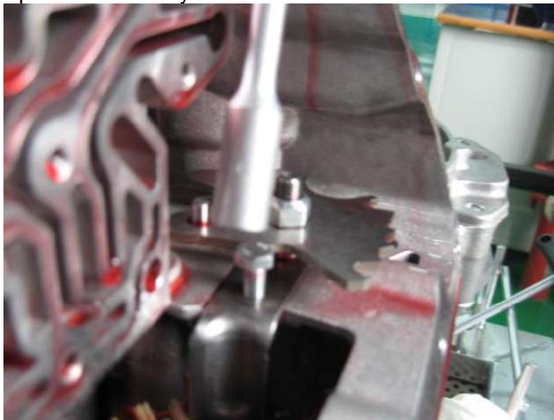
Fig. 13-1: Loosen bolt bracket output speed sensor
