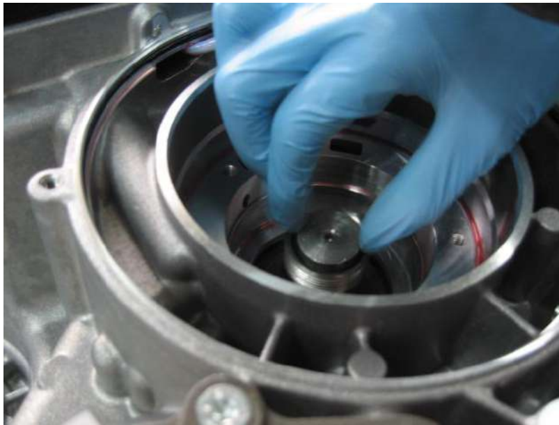
Fig. 7-3: Put special tool on shaft (primary plug 480139)
