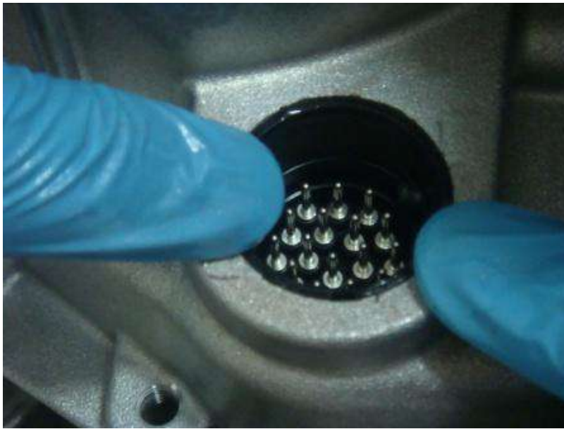
Fig. 15-2: Push main connector into the transmission
