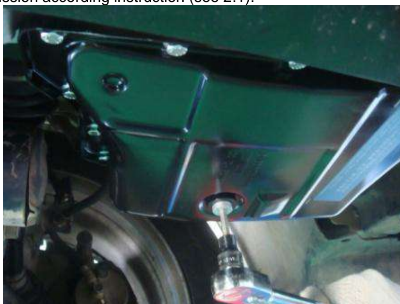
Fig. 9-1 Remove oil drain plug
