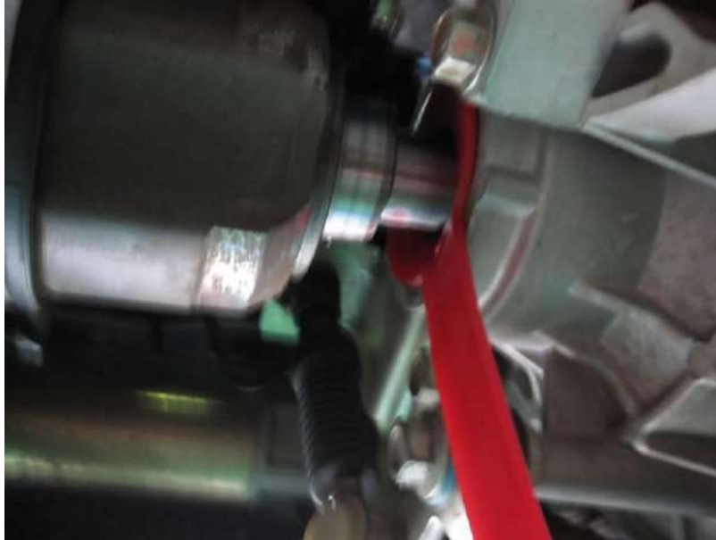
Fig. 1-3: Drive shaft inserted for 4cm
