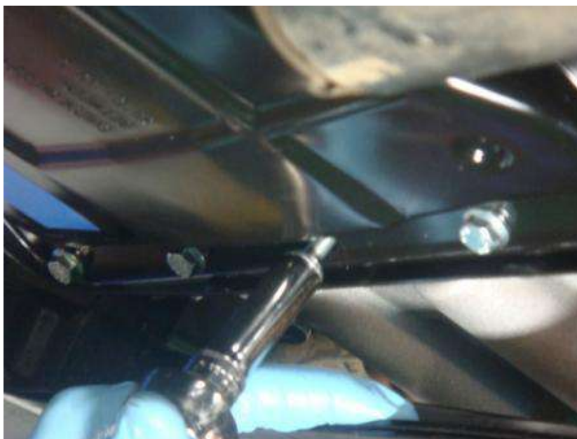
Fig. 9-2 Removing the oil pan
