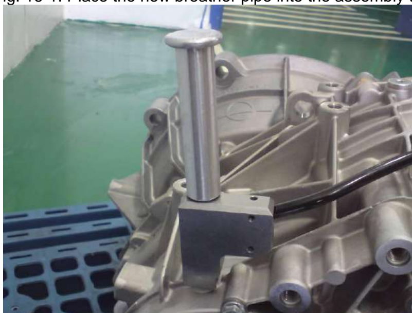
Fig. 16-2: Hammer down the tool till the end with plastic hammer
