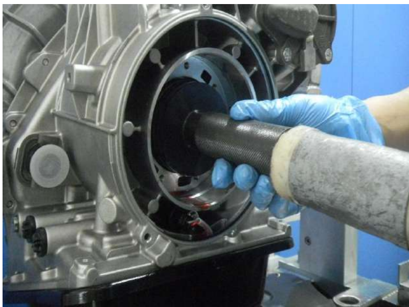
Fig. 7-7: Fit new primary ball bearing
