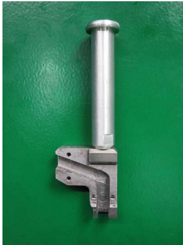
Assembly tool – breather pipe (drawing 480140)
