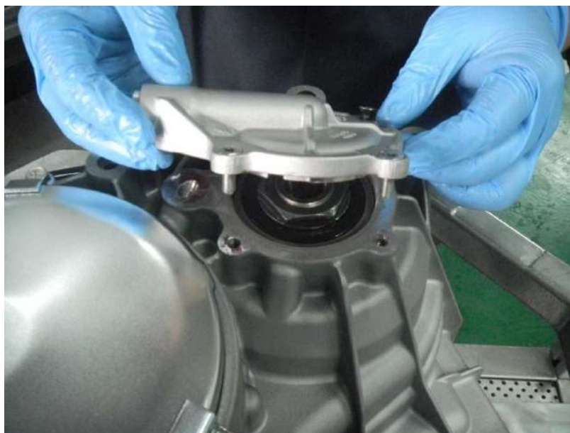
Fig.2 : remove secondary cover
