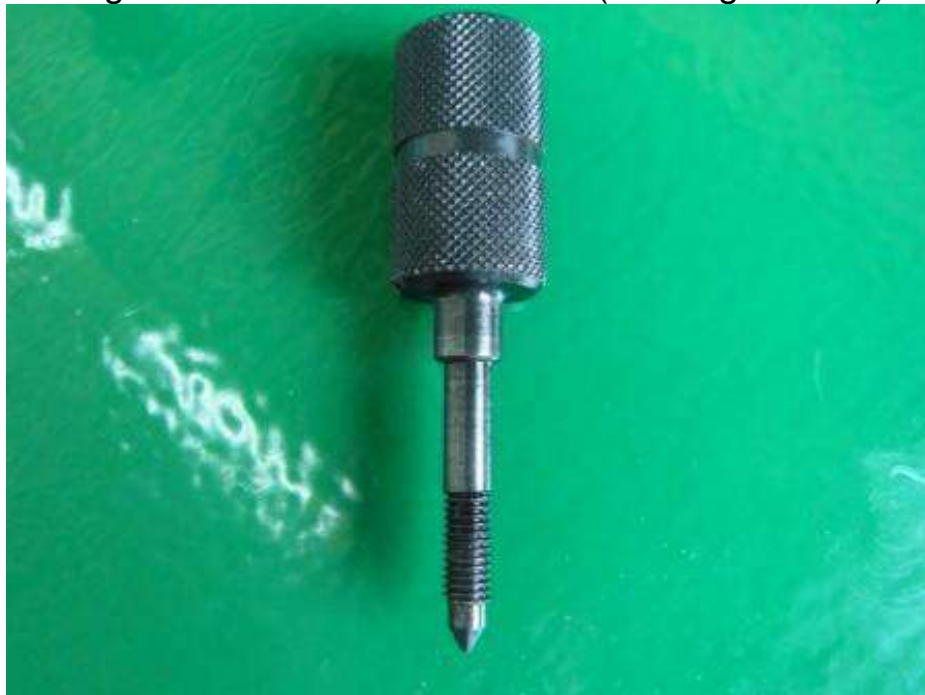
Centering pin – hydraulic unit (drawing 480142)
