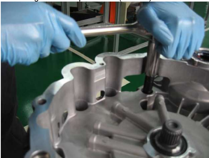
Fig. 4-2: Press and screw tool clockwise
