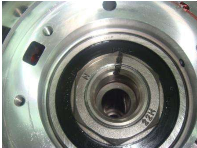
Fig. 7-1: Mark primary nut and shaft
