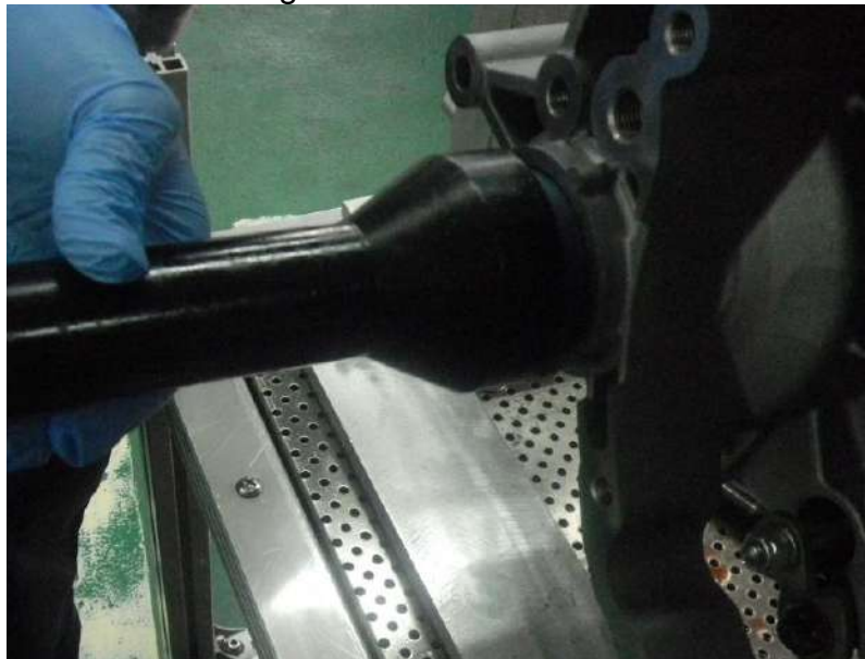
Fig. 2-2: Installing new seal with special tool
