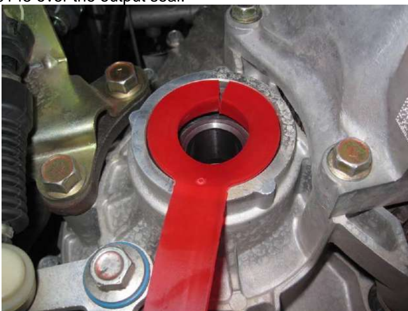
Fig. 1-2: Assembly tool drive shaft 480145 mounted
