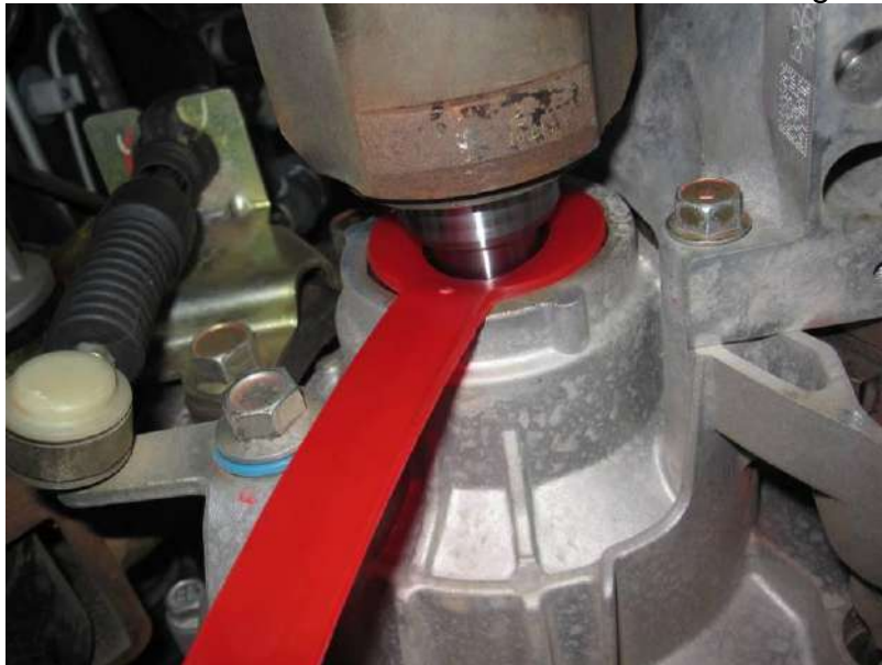
Fig. 1-4: 2 cm distance between drive shaft and tool 480145
