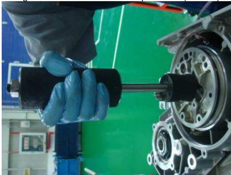
Fig. 6-2: Pull the tool to lift out pump
