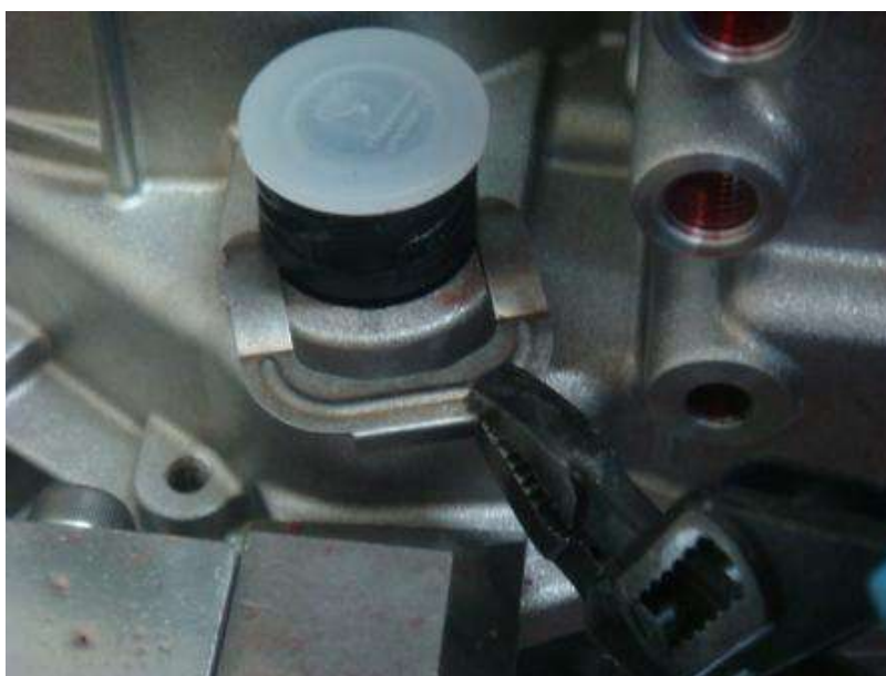
Fig. 15-1: Remove the clip from the main connector
