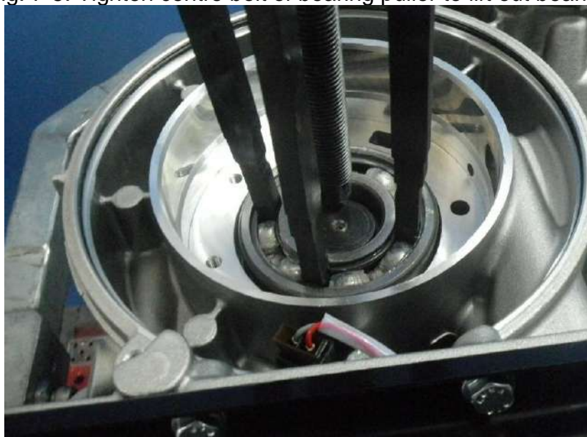
Fig. 7-6: Remove primary bearing
