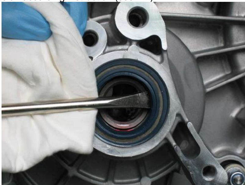
Fig. 2-1: Remove oil seal
