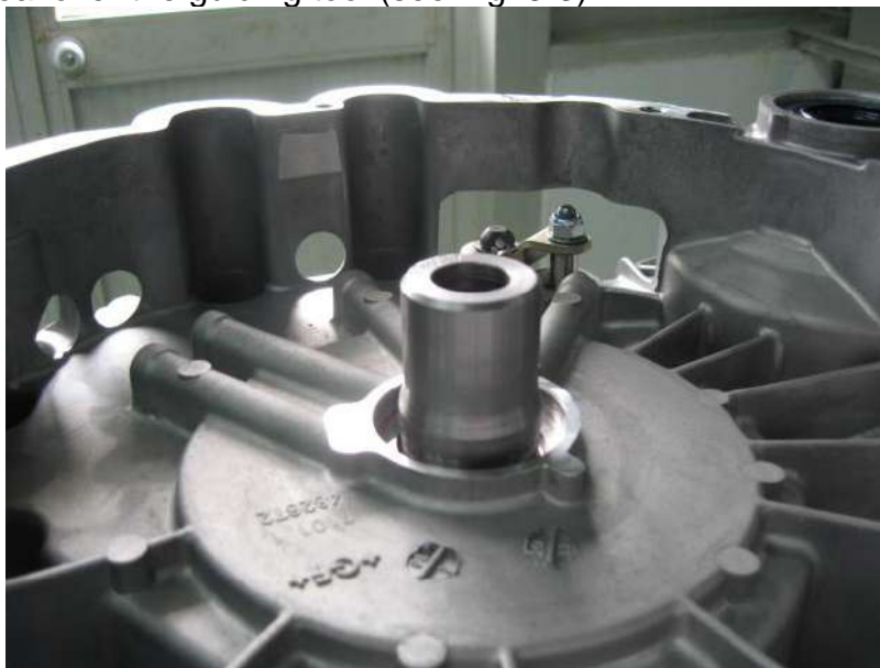
Fig. 3-2: Put special tool on input shaft (480129)
