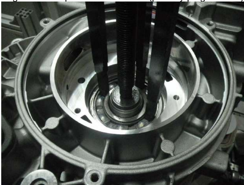
Fig. 7-4: Assemble bearing puller (480136)
