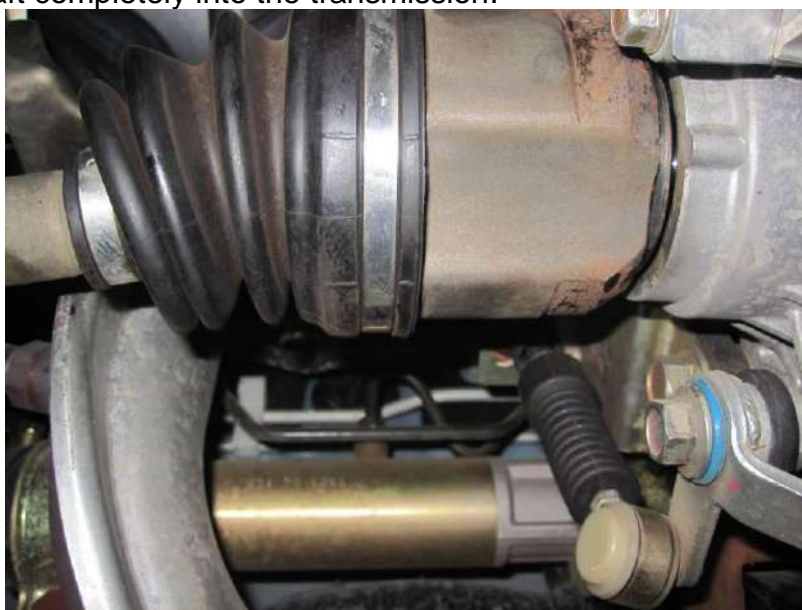
Fig. 1-6: Drive shaft mounted
