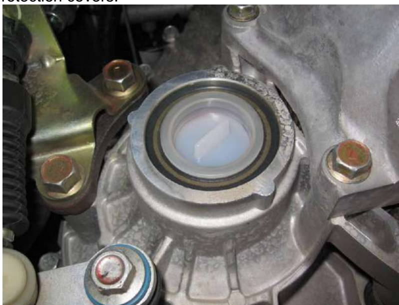
Fig. 1-1: Protective covers for differential seal
