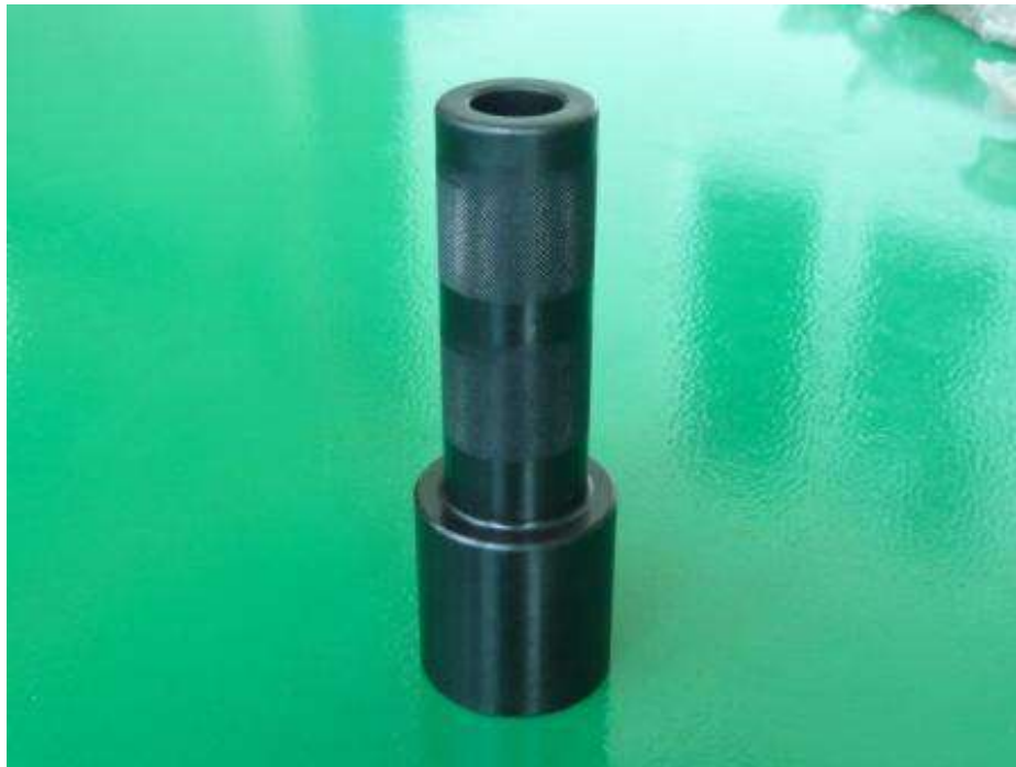
Stamp – oil seal input shaft (drawing 480130)
