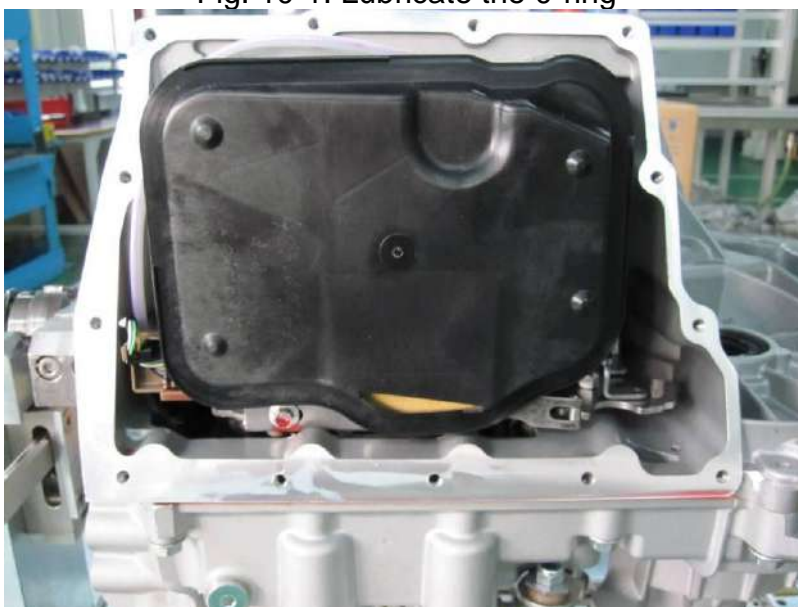
Fig. 10-2: Fix oil filter in position
