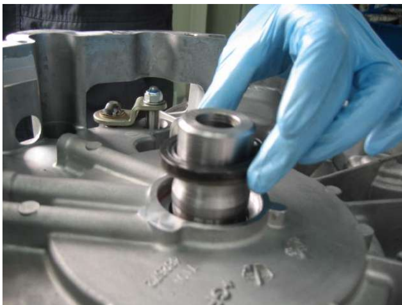
Fig. 3-3: Press the oil seal
