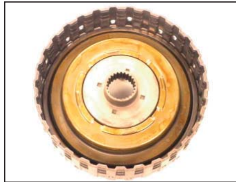
Install balance piston
