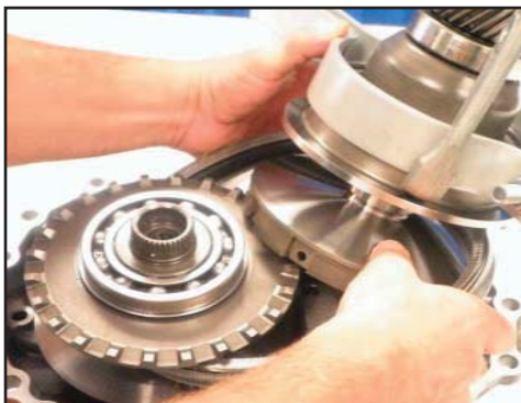
Compress secondary pulley, using new o-ring on the bolts. Torque Bolts to 33 Ft. Lbs. (45N).
