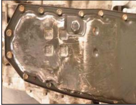
Remove the oil pan
