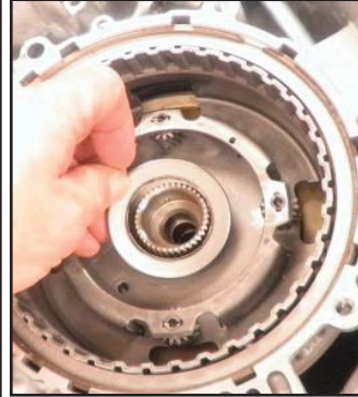
Install torrrington bearing and sun gear into planet carrier
