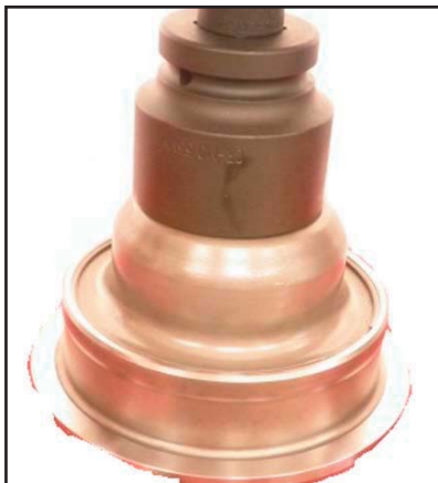
Compress balance piston
