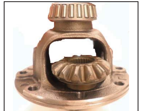
Remove both side gears and washers
