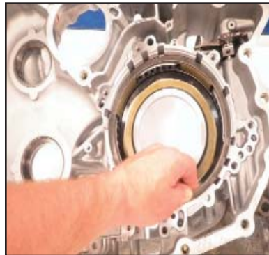
Install cushion plate, dish up
