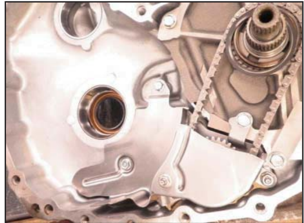
Remove o-ring, selective washer and upper baffle
