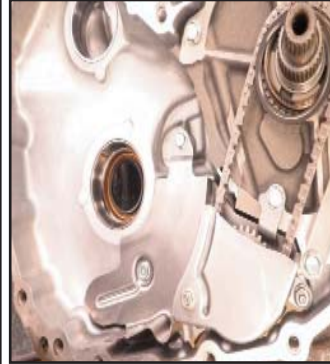
Install upper baffle. Torque to 52 In. Lbs.
