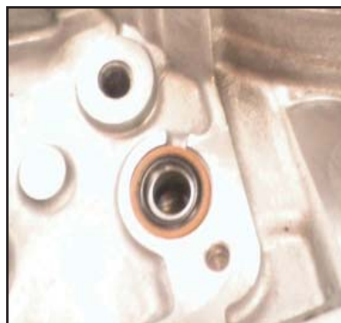
Install new pump seal, install the pump, Torque the inside bolts to 14 Ft. Lbs (19Nm) and outside bolt with o-ring to 20 Ft. Lbs (28Nm)
