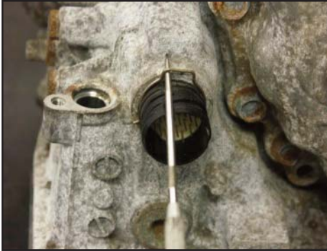
Remove clip holding in case center
