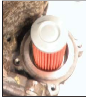
Install cooler filter
