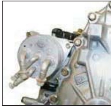
Install cooler with new o-ring. Torque bolts to 37 In. Lbs. (4Nm)
