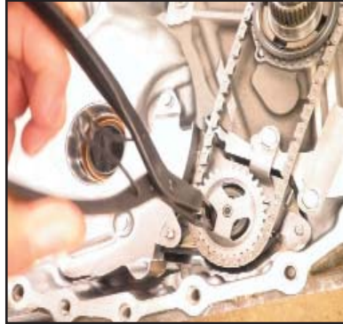
Install pump chain and gears
