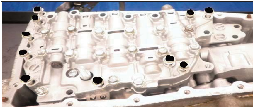
Remove marked bolts to remove valve body.
