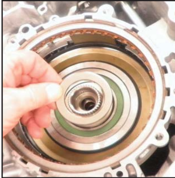
Install torrrington bearing and planet carrier
