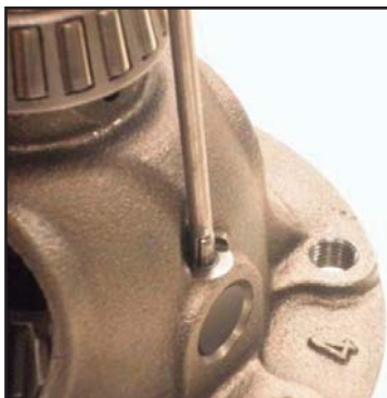
Install roll pin
