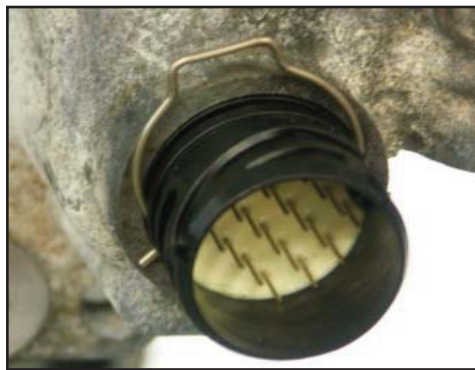
Install case connector clip
