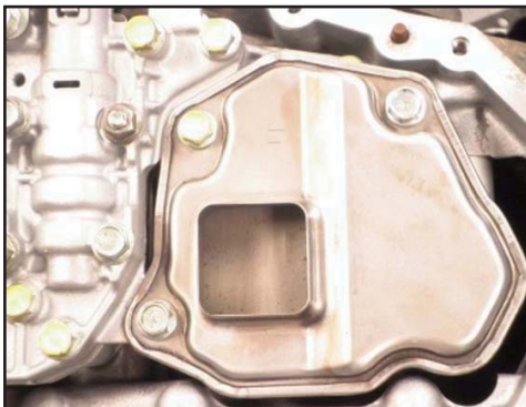
Remove the filter
