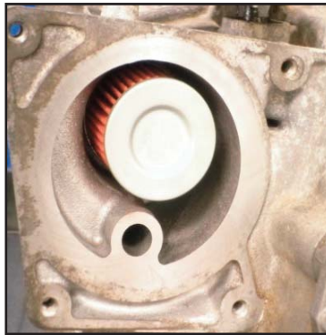
Install cooler filter
