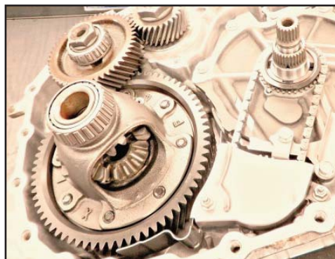
Install differential and transfer gears
