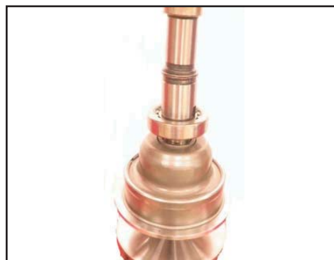
Press secondary piston down just enough to install the piston retaining snap ring. You may need to tap the balance piston down to get the snap ring in. Once the snap ring is installed, continue pressing the piston until it is completely seated.
