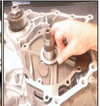
Install stator support and thrust washer
