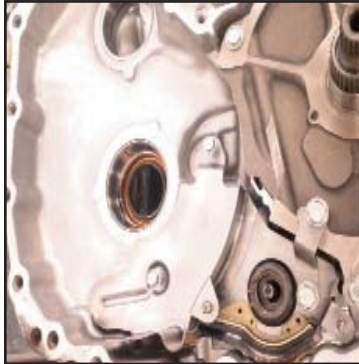
Install lower oil baffle and pump bracket. Torque baffle bolts 52 In. Lbs. Pump bracket and stator support bolts to 19 Ft. Lbs.
