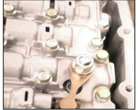
Remove the manual lever
