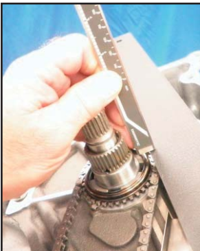
Measurement A from straight edge to the Measurement B step on gear. To calculate the correct shim. A + B - .0065\text{in. (.16mm)}
