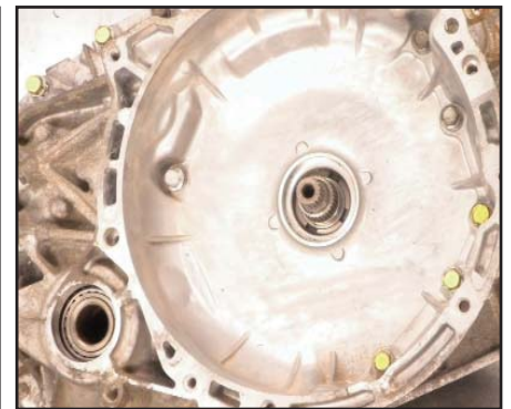
Using loctite 509 sealer, install the bell housing bolts marked in yellow. Torque to 33 Ft. Lbs. (45Nm). Bolts marked in yellow 1.67 in(42.8mm)
