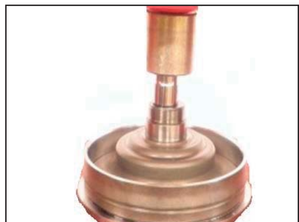
Press the pulley halves apart. Place a container under the press, there are six 6mm balls that will be saved.
