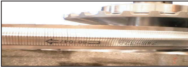
Note the direction of the belt
