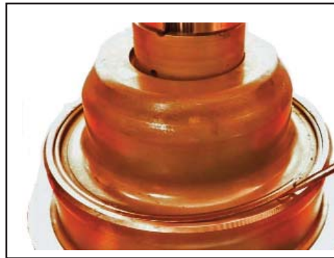
Press secondary piston down just enough to install the piston retaining snap ring. You may need to tap the balance piston down to get the snap ring in. Once the snap ring is installed, continue pressing the piston until it is completely seated.
