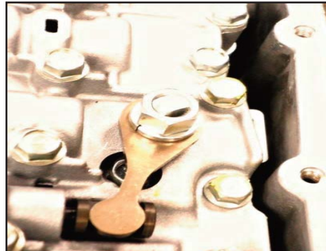
Install manual lever onto manual shaft. Tighten nut to 194 In. Lbs. (22Nm)
