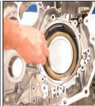
Install steel plate then friction plate, alternating ending with friction plate.
