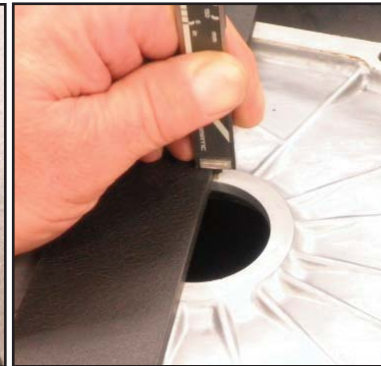
Measurement A from straight edge to the Measurement B step on gear. To calculate the correct shim. A + B - .0065\text{in. (.16mm)}
