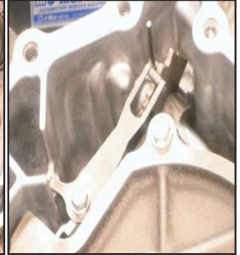
Install pin for manual valve shaft and detent spring. Torque bolt to 61 In. Lbs.
