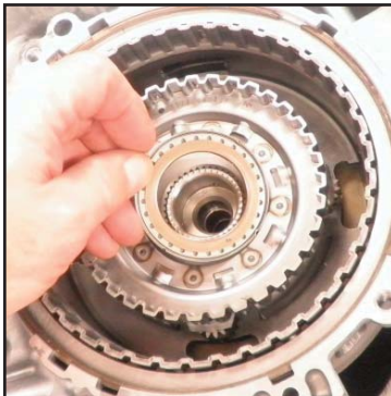
Install torrrington bearing
