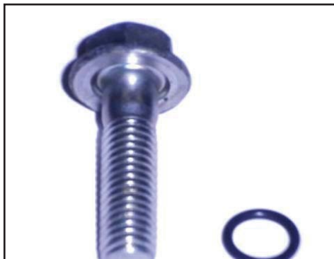
Compress secondary pulley, using new o-ring on the bolts. Torque Bolts to 33 Ft. Lbs. (45N).
