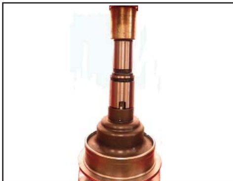
Press secondary piston down just enough to install the piston retaining snap ring. You may need to tap the balance piston down to get the snap ring in. Once the snap ring is installed, continue pressing the piston until it is completely seated.
