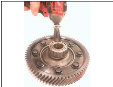
Remove ring gear
