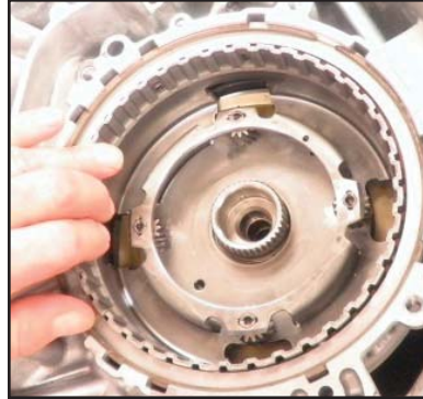
Install torrrington bearing and planet carrier
