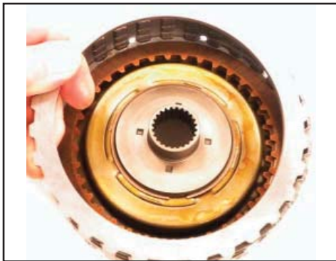
Install forward clutch pressure plate
