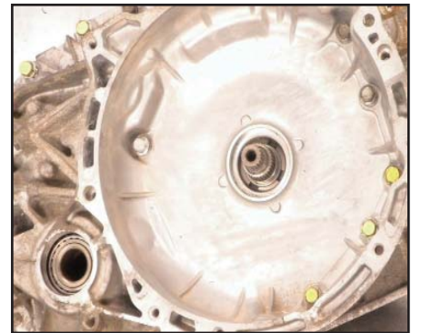
Remove bell housing bolts.
