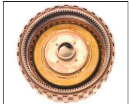
Start with steel plate, then friction plate, alternating ending with a friction plate
