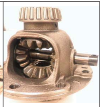
Install spider gear shaft
