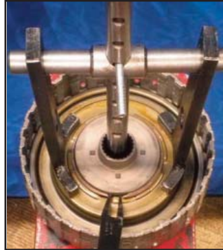
Compress the retainer and remove snap ring
