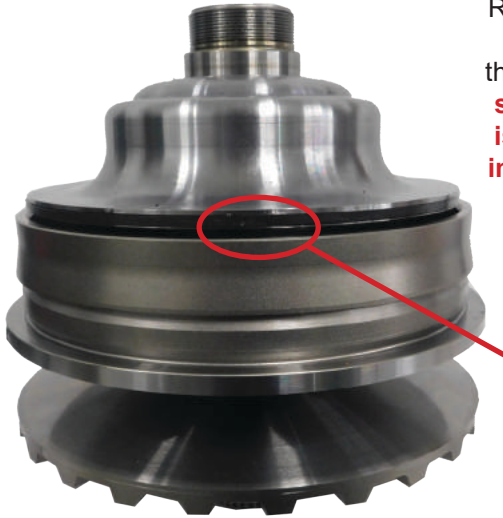
Stepped lap joint in sealing ring in the apply piston.
