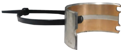
4L80E Tail Housing Bushing Cut In Half
