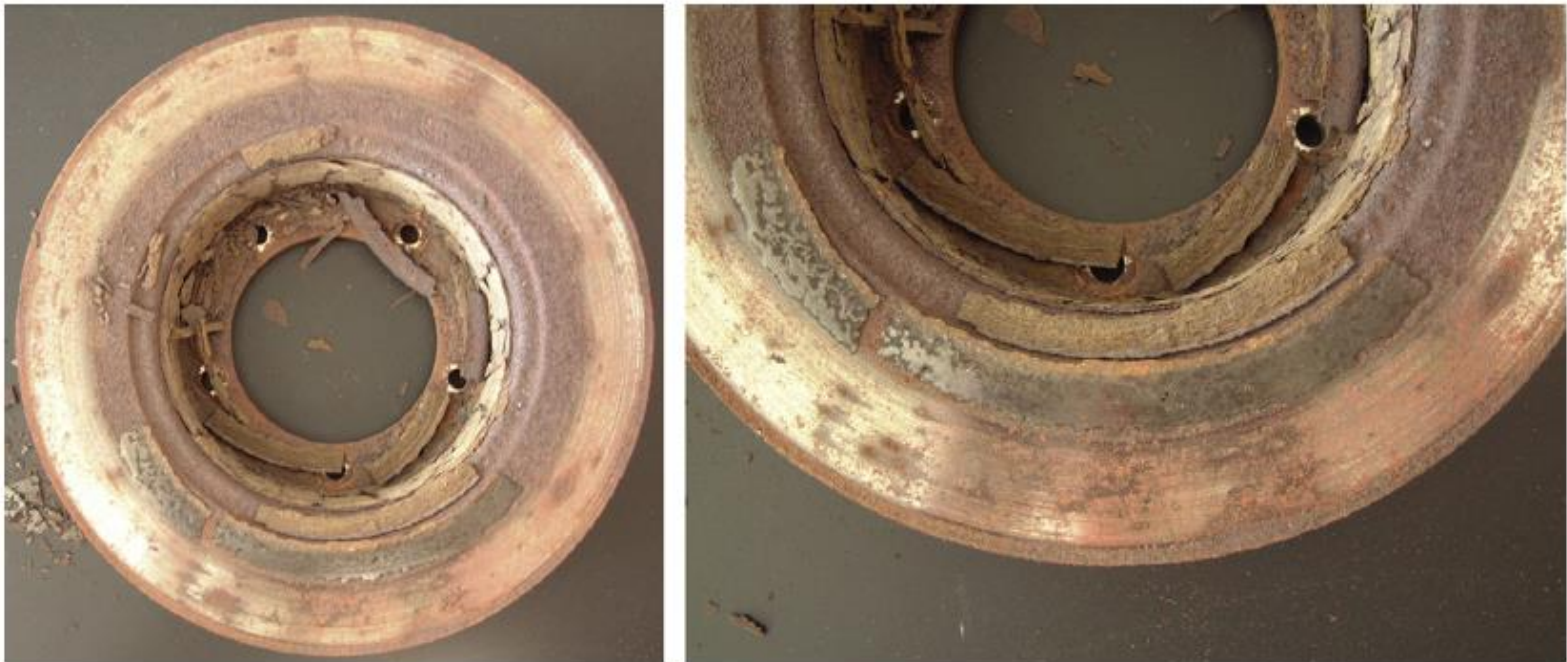
Figure 12.3: Corroded Brake Disc.
