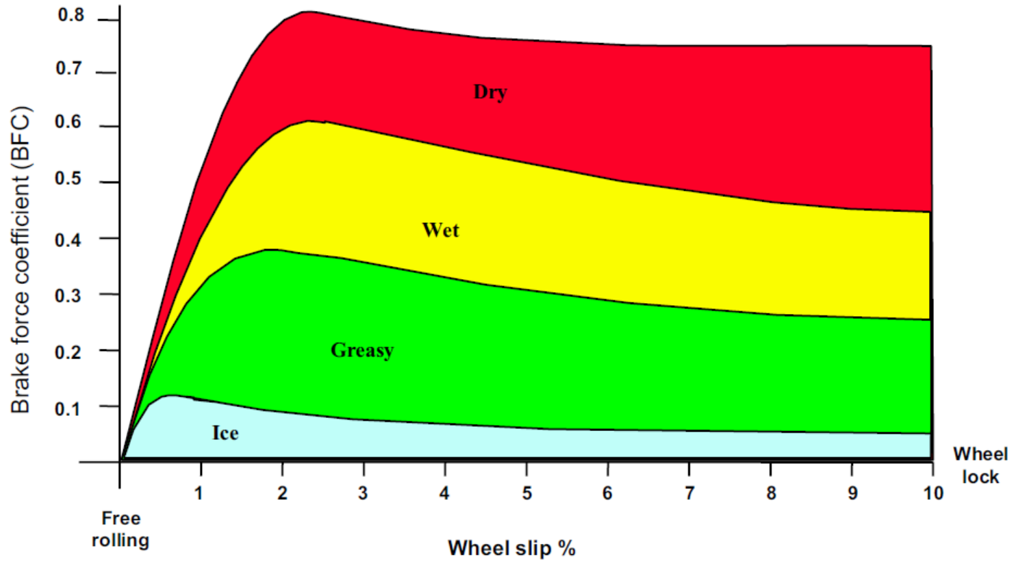
Figure 11.2: Brake Force Coefficient (BFC) vs. Wheel Slip: Example Characteristics for Different Road Surfaces (Ross, 2013).
