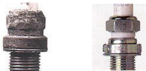
Rust The Caulked Portion
