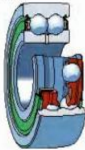
Cam roller, wide design
