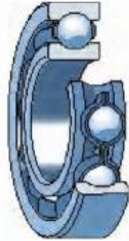
Deep groove ball bearing, open basic design
