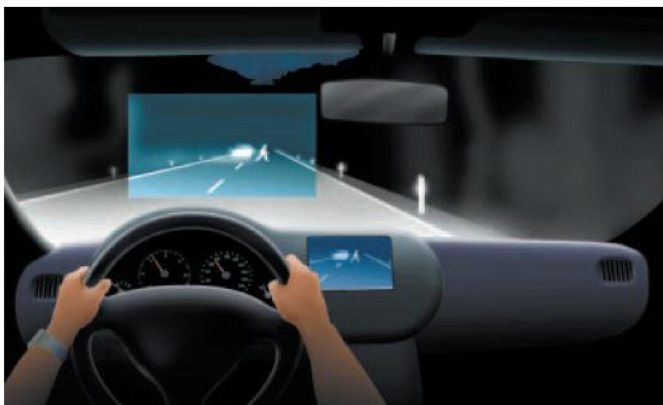
Presentation of the camera picture on a Head-Up-Display/Dashboard-Display
