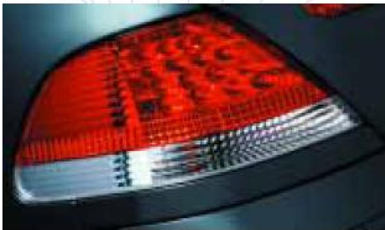
The BMW 7-series has a total of 74 LEDs in the rear-end.
