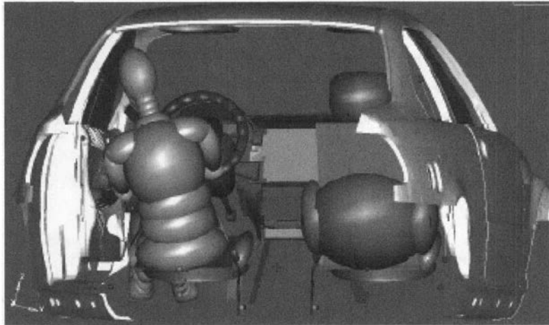
Figure 5.27 An occupant model position 30 ms after head-to-side-window contact. (Praxl et al. , 2003.)
