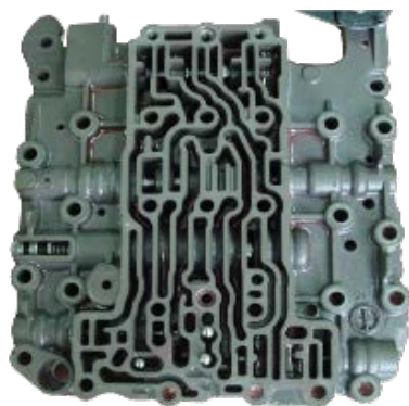
Inside valve body (MS)
