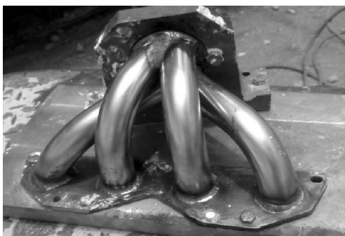
Fig 1. Under construction exhaust manifold sample.
