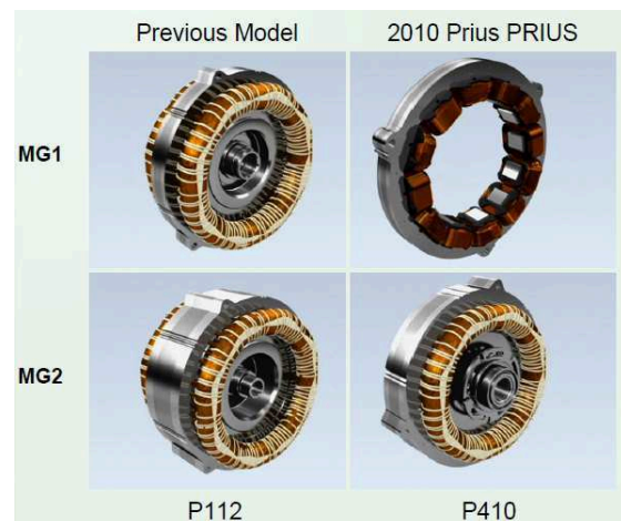
Fig. 8. Two generations of the electric machines MG1 and MG2
